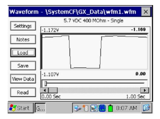
Waveprints are very useful with regard to confirming switching synchronization of current interrupters, for example, and with regard to checking for On-to-Off and Off-to-On transition spikes.
