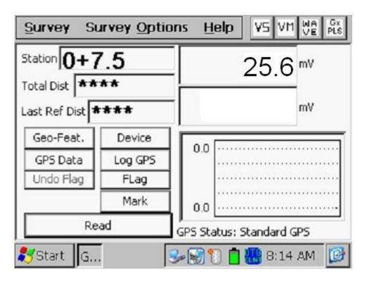
*Note:* When readings are logged, the latest logged reading (the prior reading) is displayed in the bottom mV field on the above screen and the current reading is displayed in the top mV field (see the screen below for an example).
