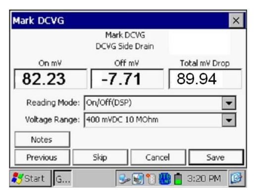
The "Mark DCVG" device will not appear in the Device list if this box is not checked, which would be the case if you were conducting a regular CIS.
