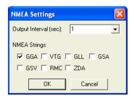
The NMEA data string format labeled as, "GGA" should be selected (box checked). All other boxes should be left unchecked.
