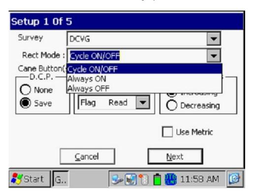
As can be seen from the above screen, there are 3 choices for "Rectifier Mode". However, only the "Cycle On/Off" option should be selected for DCVG surveys, as rectifier current interruption is a requirement for this survey type.
