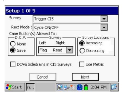
Step 5: Select the survey type by tapping on the menu button in the "Survey Type" field and highlighting the survey type of your choice.
