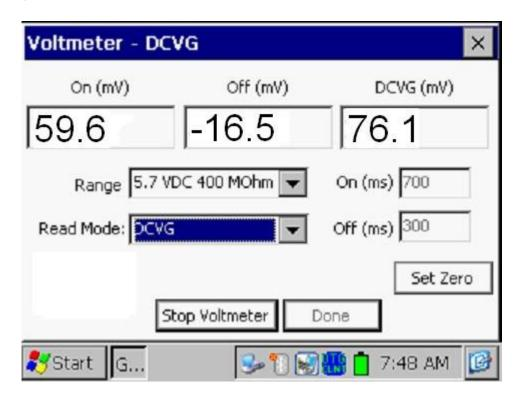
As can be seen from the above screen, the delta V(ON) reading is +59.6mV and the delta V(OFF) reading is -16.5mV. Consequently, the DCVG voltage is 76.1mV.
