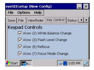
White Balance – (numeric "2") cycles through the color (white) balance modes advancing one selection with each key press.
