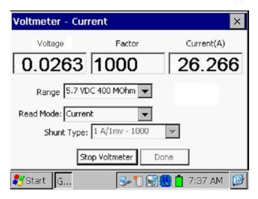
A number of industry standard shunts can be selected by tapping on the menu button in the "**Shunt Type**" field, after tapping on the "Stop Voltmeter" button to make any desired settings changes. You can also select "other" and enter your own shunt factor in the "Factor" field.
