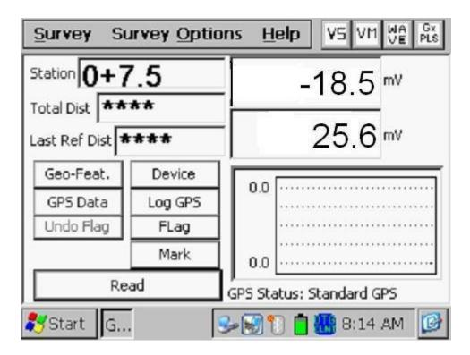
On the above example screen, the prior reading was 25.6mV and the current reading is -18.5mV. In this example, a polarity switch has been detected, which means that a gradient field has been detected.
