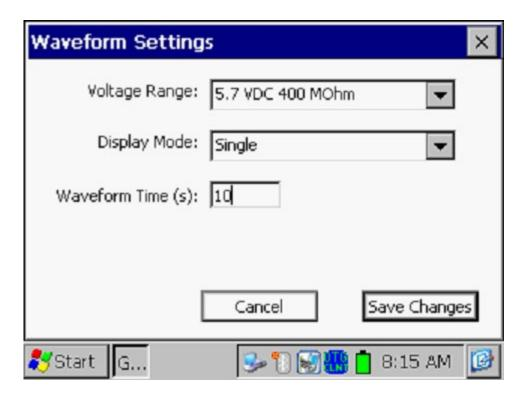
Since all of the DC channels on the Gx data-logger are fast response channels, you can select any "Voltage Range" setting amongst the DC options, regardless of the interruption cycle rate. The main issue with regard to optimum Range selection is sensitivity, in terms of the magnitude of the voltages being measured.
