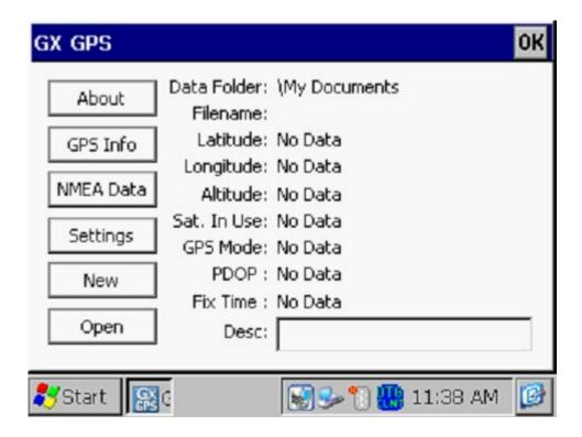
The data parameters are self-explanatory with the exception of the PDOP parameter. This acronym stands for, Position Dilution of Precision. These data provide position accuracy information.
