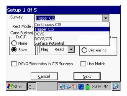
For Close Interval (Potential) Surveys there are 2 options for "type of survey": Trigger CIS and Continuous CIS.
