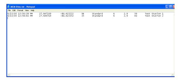
From left to right, the data displayed are: date, time of position fix, latitude, longitude, altitude, GPS status (standard or differentially-corrected), number of satellites in use, the PDOP and, finally, the description of the location (provided by you).
